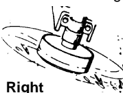
Tip of the Line Does The Cutting
